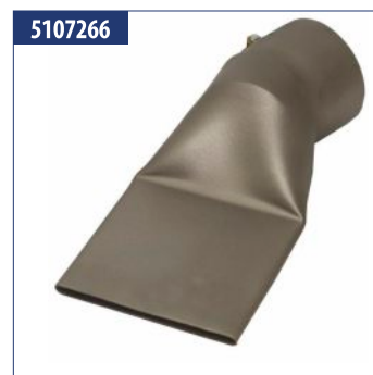
Nozzles for hot-air blower ERON: Wide slot nozzle 70 x 2 mm (bitumen nozzle), push-fit (with device holder)
