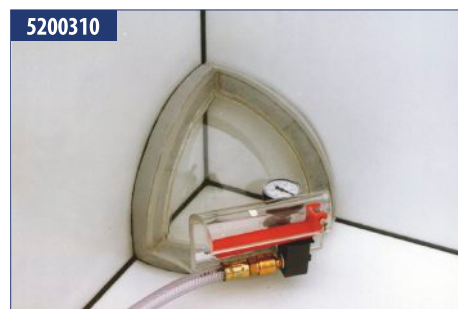
Testing bell Inside corner, bottom 1/8
